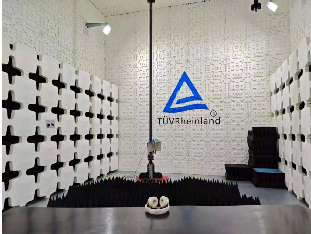
Photograph 3: Set-up for Radiated Emission, above 1GHz
