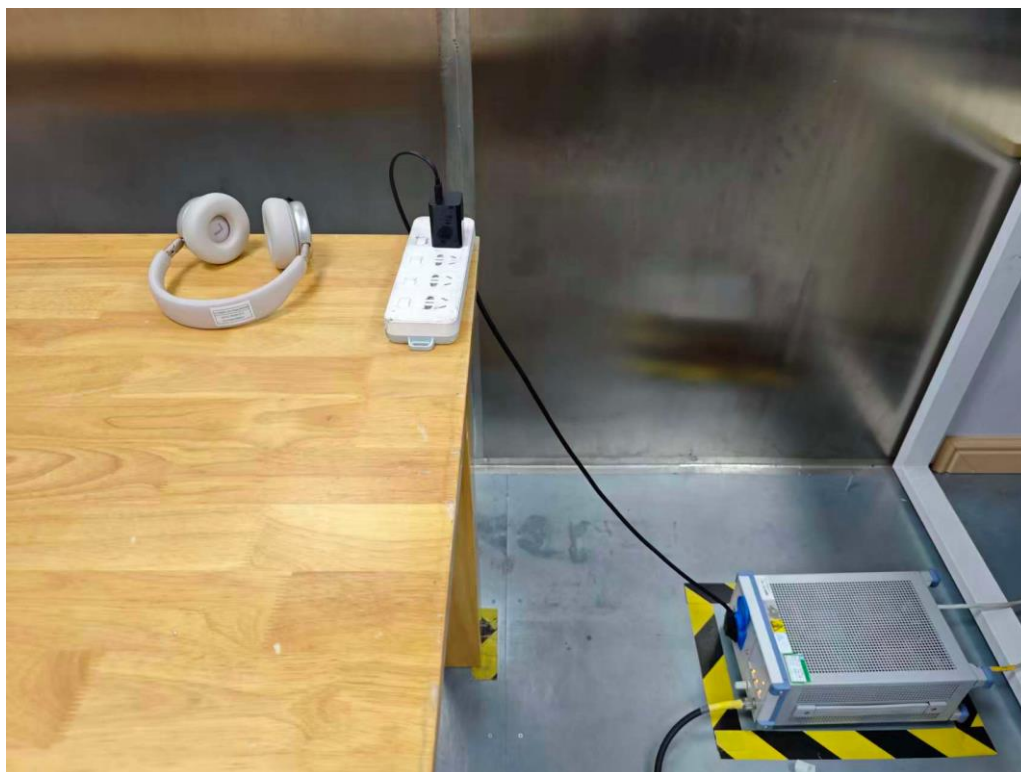
Photograph 2: Set-up for Radiated Emission, below 1GHz
